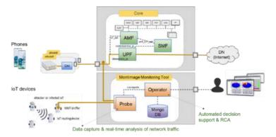
networks, including 4G/5G and IoT mobile networks ranging from physical to application network layers, business activity, and manufacturing processes. It includes intrusion detection and prevention (MMT-Probe), Cyber Threat Intelligence services (Cartimia), Root Cause Analysis (MMT-RCA), IoT sniffing (MMT-IoT), and pentesting/training tools (MI Cyberrange).
